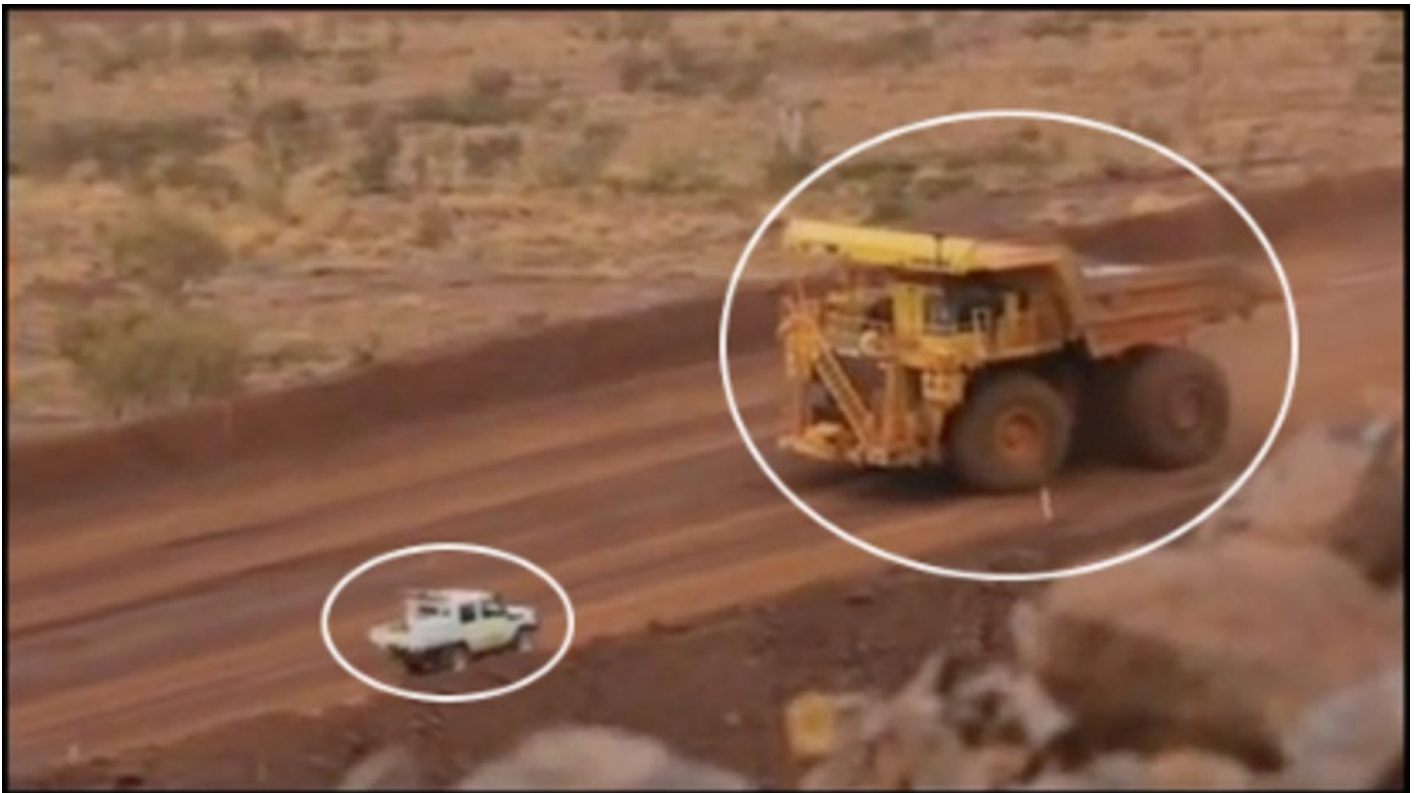
The Komatsu AHS (right) is an autonomous earth moving machine
